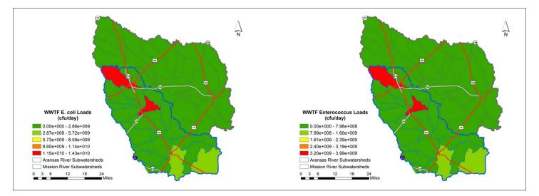
Figure 33. Potential *E. coli* and *Enterococcus* loads resulting from wastewater treatment facilities (WWTFs) for the Mission and Aransas rivers watersheds.
