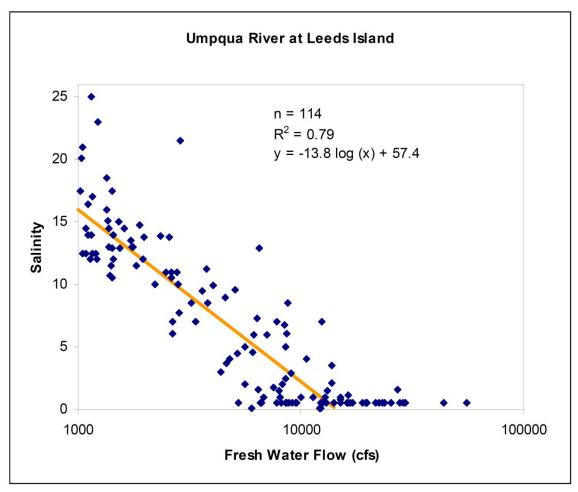
Figure 40. Example salinity to flow regression from Umpqua Basin tidal streams (ODEQ 2006).
