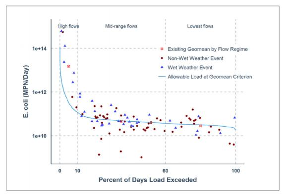
Figure 22. Load duration curve for Aransas River Above Tidal surface water quality monitoring station 12952.
