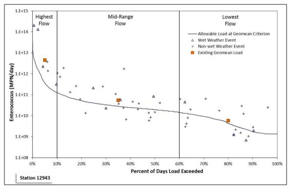
Figure 20. Load duration curve for Mission River Tidal surface water quality monitoring station 12943.
