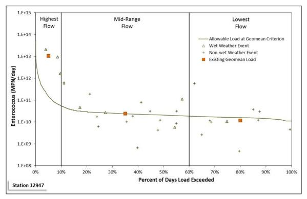
Figure 21. Load duration curve for Aransas River Tidal surface water quality monitoring station 12947.
