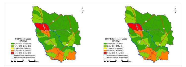
Figure 31. Potential *E. coli* and *Enterococcus* loads resulting from on-site sewage facilities for the Mission and Aransas rivers watersheds.
