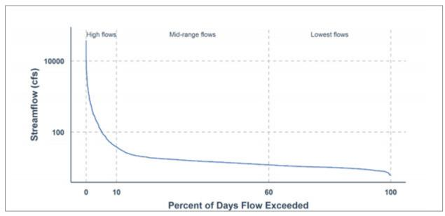
Figure 43. Flow duration curve for station 12952, Aransas River Above Tidal.
